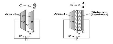
Fig. 2.3 Parallel Plate Capacitors
