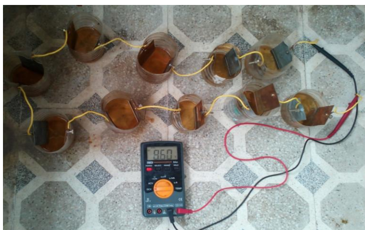
Figure 3(b) shows actual practical set up of cow urine power generated system
