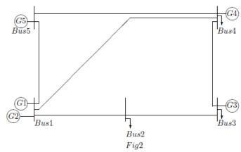
Loads are inelastic and are 300MW each. Bus 4 is taken as the slack bus.
