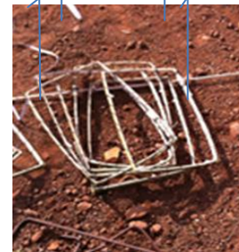
Fig. No. 6 Bamboo Stirrups of Bamboo
