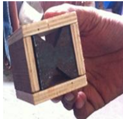
Fig. No.4 triangular blocks for shear test
