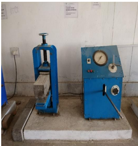
Fig. 5. Flexural Strength Testing of specimen
