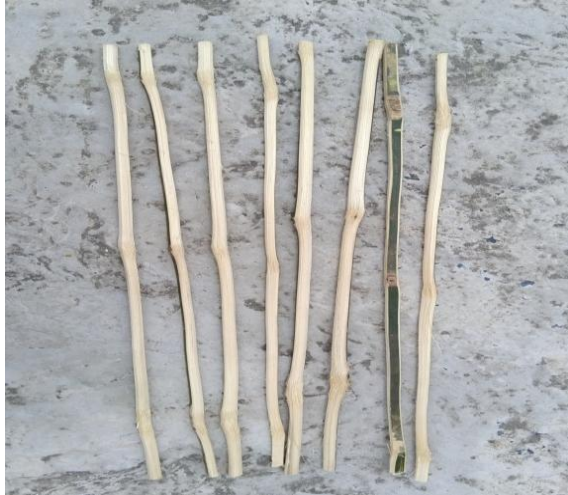
Fig.1. Longitudinal reinforcement made up of green bamboo of 12mm
