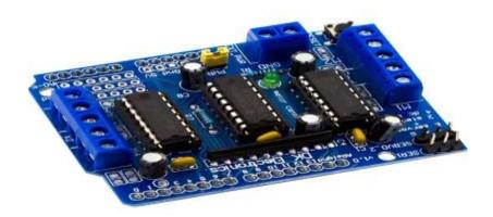
The L293D is a dual-channal H-bridge motor driver. It can control two DC motors or a stepper motor at one time. It is technically capable of controlling a total of four DC motors.
