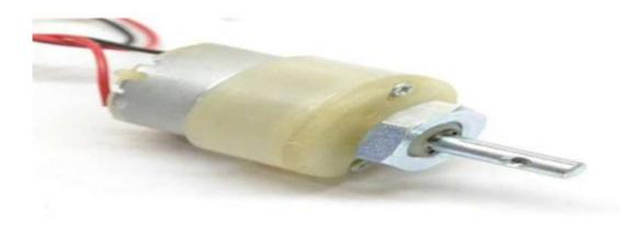
DC Motor – 12volts geared motors are generally a simple DC motor with gearbox attached to it. This can be used in all-terrain robots and a variety of robotic applications. These motors have a 3mm threaded drill hole in the middle of the shaft thus making it simple to connect it to the wheel or any other mechanical assembly. 12V DC geared motors widely use for robotics applications.
