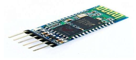
HC-05 Bluetooth Module is an easy- to- use Bluetooth SPP (serial port protocol) module, designed for transparent wireless serial connection setup. HC-05 Bluetooth module provides switching mode between master and slave mode which means it able to use neither nor transmitting data.
